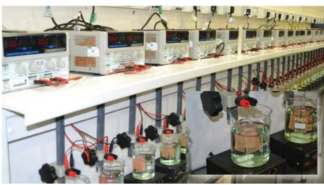
The electrolysis area in full operation (Inset: During electrolysis the copper deposits from the test solution onto a platinum mesh)
